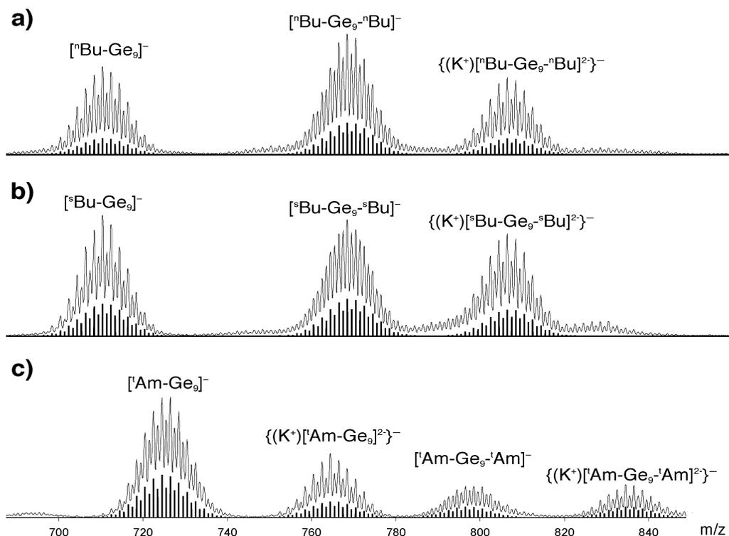
**Figure 3.** Electrospray mass spectra (negative-ion mode) of the reaction mixtures of ethylenediamine solutions of  $\text{K}_4\text{Ge}_9$  reacted with: (a)  ${}^n\text{BuCl}$ , (b)  ${}^i\text{BuCl}$ , and (c)  ${}^t\text{AmCl}$ . Shown under each peak is the calculated isotope distribution for the corresponding ion. The spectrum of the reaction with  ${}^i\text{BuCl}$  (in Supporting Information) is virtually identical with those seen in a and b.
